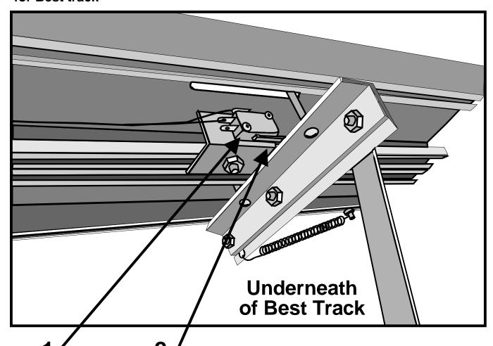
Micro Switch Bolt micro switch to "L" Bracket
