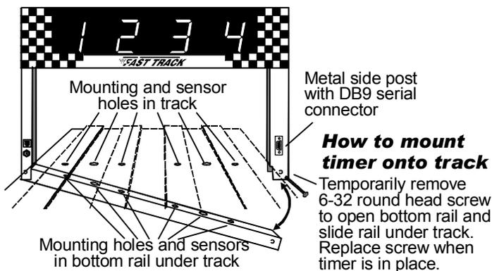
Once these holes are drilled, you are ready to mount the Fast Track finish line to your track. Remove the screw in the bottom corner of the finish line opposite the power jack. With this screw removed, the finish line can now hinge open. (If you remove the wrong screw, it can't be opened due to the wires running to the sensors). Remove and save the 2 mounting screws.
