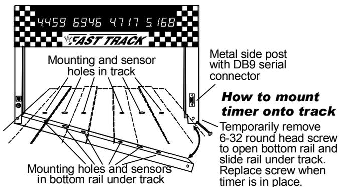
Once these holes are drilled, you are ready to mount the Fast Track finish line to your track. Remove the screw in the bottom corner of the finish line opposite the power jack. With this screw removed, the finish line can hinge open. (If you remove the wrong screw, it can't be opened due to the wires running to the sensors). Remove and save the 2 mounting screws.
